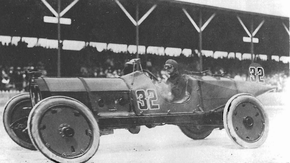
Ray Harroun wins the first 500, aided by what is believed to have been the very first rearview mirror ever used on an automobile. It's on rods above the cowling.
